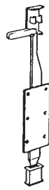
No. 77J Flush Bolt for bottom rail up to 152 x 48 on framed and ledged door
